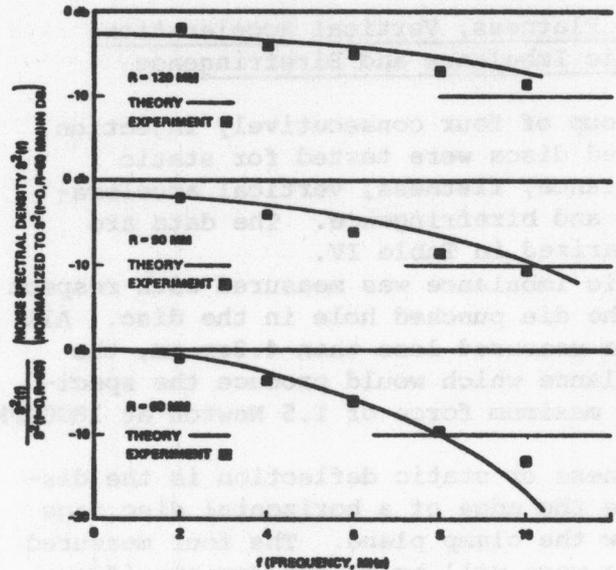
FIG. A-1. THEORETICAL AND MEASURED NOISE SPECTRAL DENSITY FOR A DISC OF RANDOMLY VARYING REFLECTIVITY.  $\lambda = 0.633$  MICRON,  $NA = 0.45$
