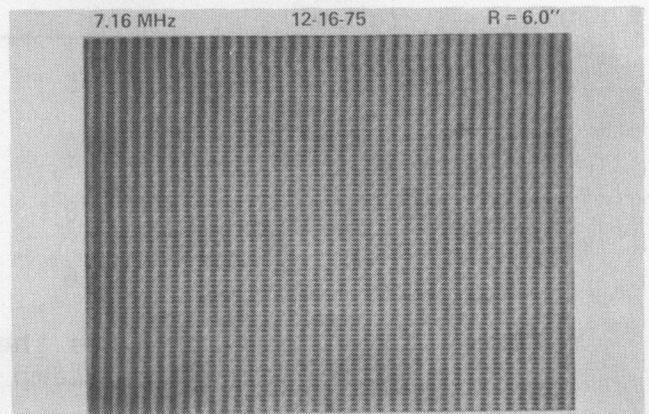
Fig. 3: Photo micrograph of master disc cut with frequency doubled color subcarrier. The track-to-track alignment implies that the rotation period of the spindle repeats itself to better than 14 nanoseconds.
