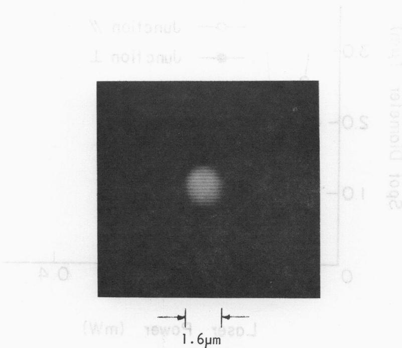
Fig. 4 Near field pattern shape of the BH laser
