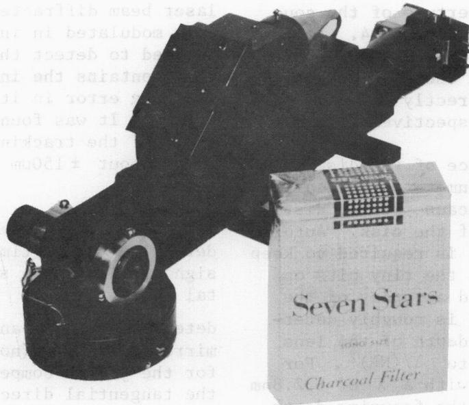
Fig. 12 Appearance of the semiconductor laser pickup.
