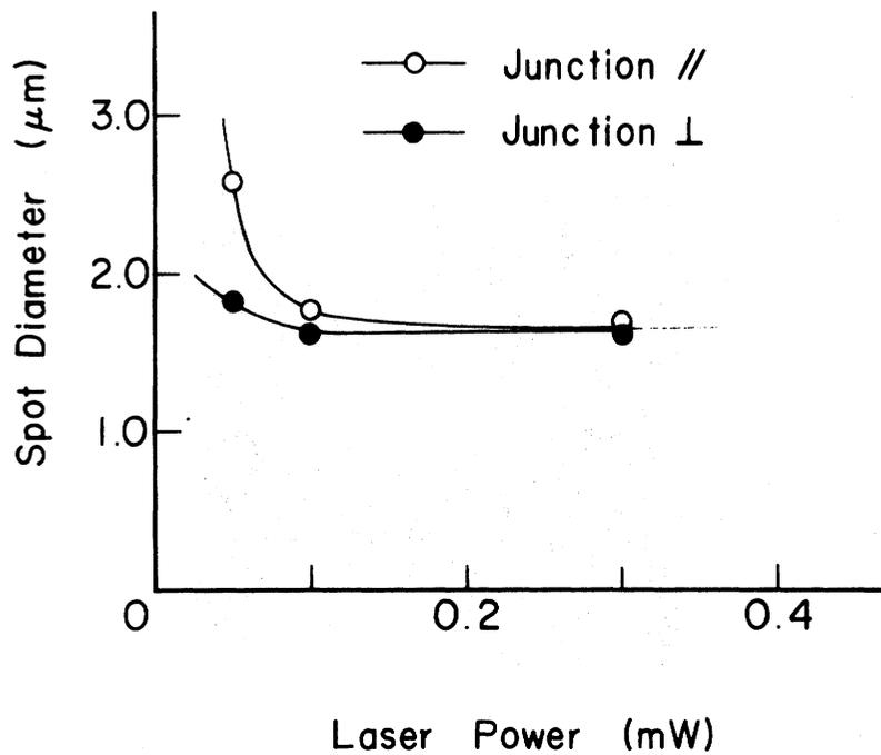
Fig. 6 Dependence of the spot size of the BH laser on the output laser power.
