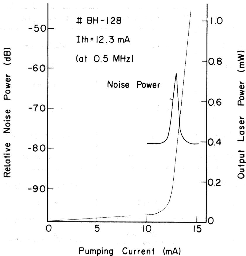
Fig. 10 Dependence of the relative noise power of the BH laser on the excitation current.
