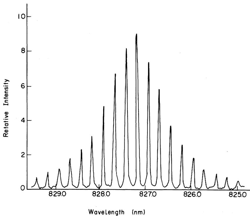
Fig. 8 Typical lasing spectrum of the BH laser
