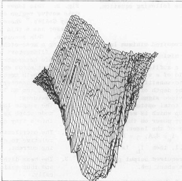
Fig. 3 3-dimensional plot of the far field pattern of the BH laser.
