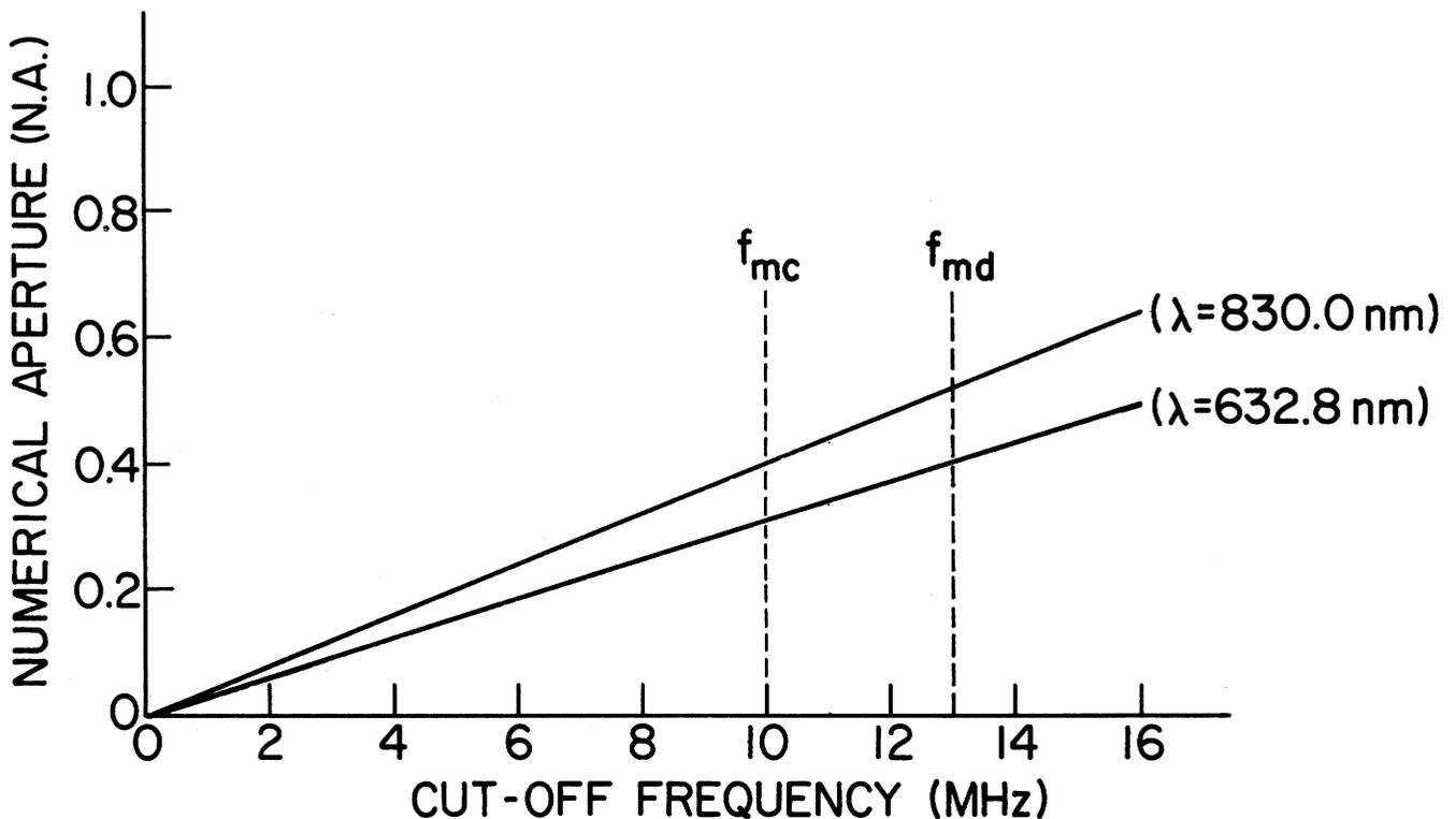
Fig. 1 Relation between the cut-off frequency and the numerical aperture of the lens.
