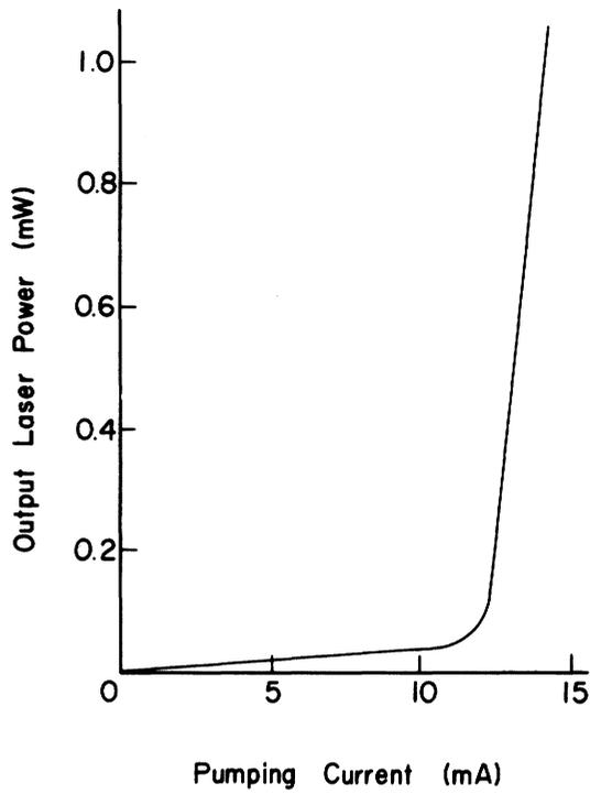
Fig. 7 Dependence of the output laser power of the BH laser on the excitation current.
