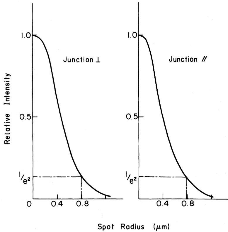
Fig. 5 Detailed cross sections of the near field pattern of the BH laser.
