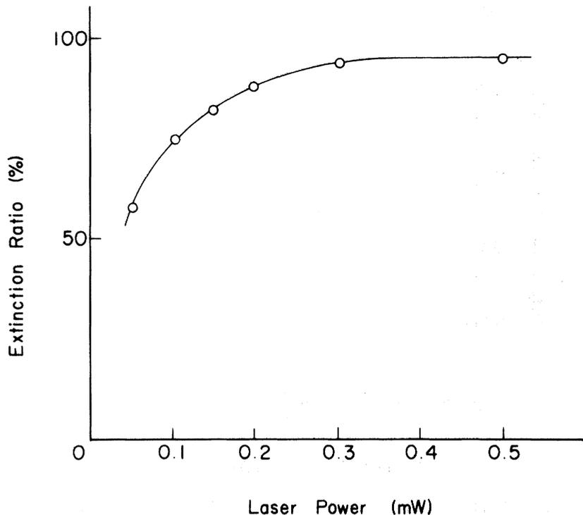
Fig. 9 Dependence of the extinction ratio of the BH laser on the output laser power
