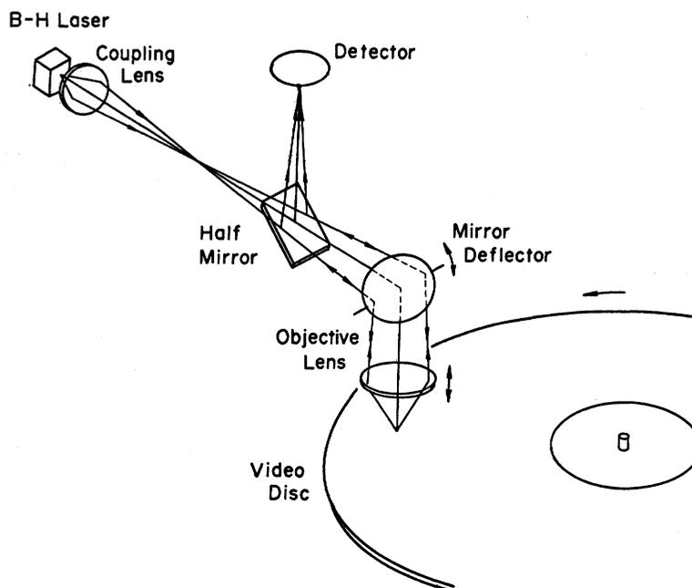
Fig. 11 Basic configuration of the semiconductor laser pickup.
