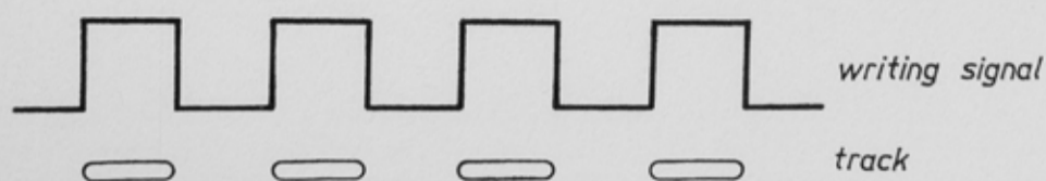
Fig. 1. The writing signal that drives the laser-beam modulator and the resulting track.
